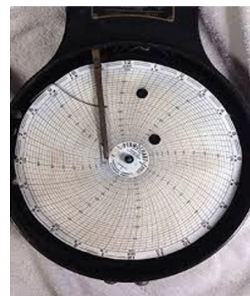
Temperature recording paper with a pen (inkless) used in the past
