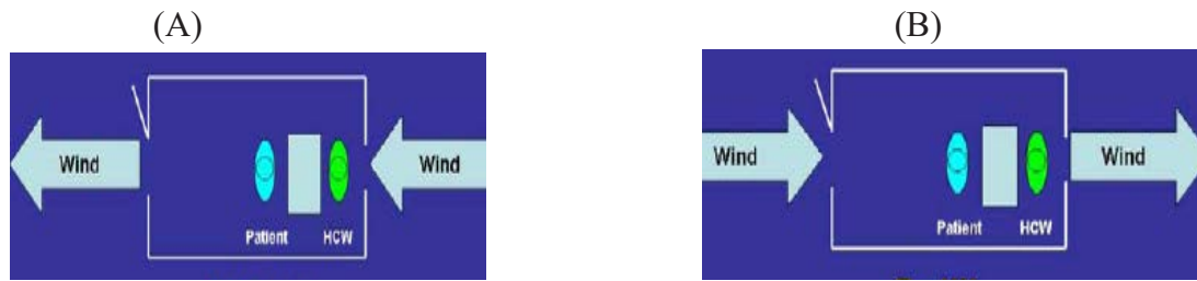
(A) Direction of natural ventilation and correct working location. (B) Direction of natural ventilation and incorrect working condition.
