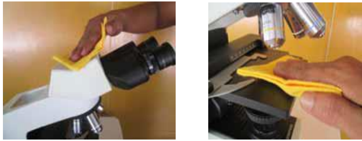
Figure 3 cleaning the body parts of the microscope
